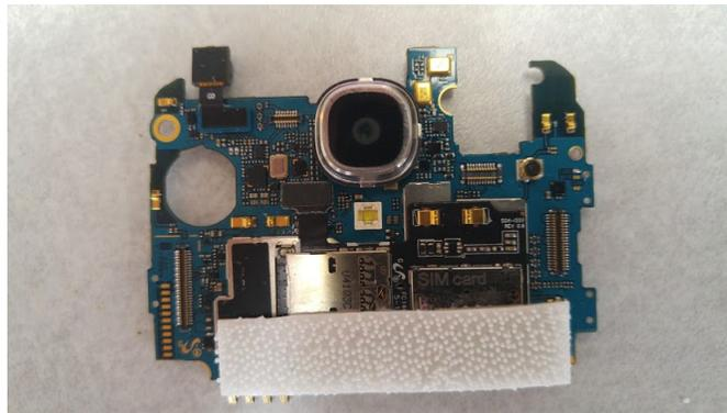
Figure 7: Chipset alone; note that the RGB light sensor, IR sensors, LED indicator, and vibration motor are missing as they were lost on impact.
