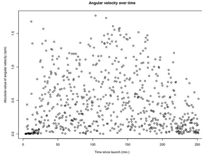
Figure 26: Angular velocity-time graph showing spinning during flight.
