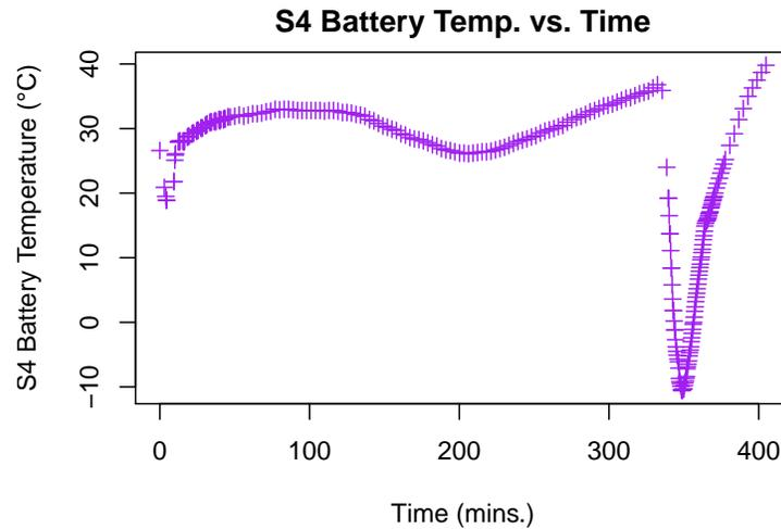
Figure 37: Battery temperature-time graph for the S4 during ECLIPSE.
