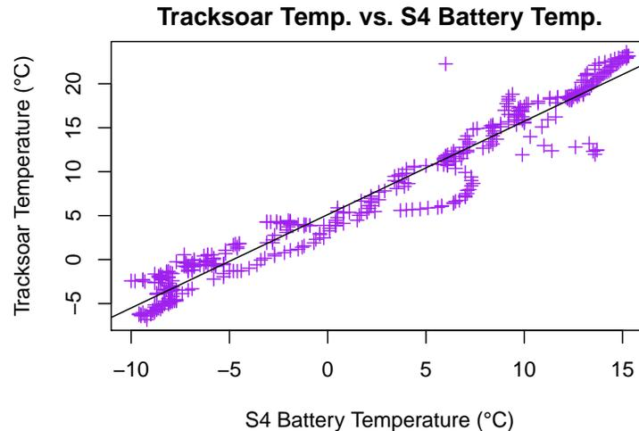
Figure 21: Temperature-temperature graph demonstrating the general correlation between the measurements of temperature by the Tracksoar and the S4 battery temperature.
