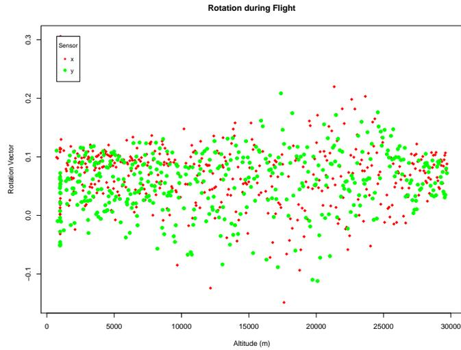
Figure 24: Rotation-altitude graph showing swinging during flight.
