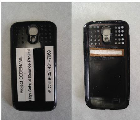
Figure 9: Plastic phone back modified to house the chipset and battery.
