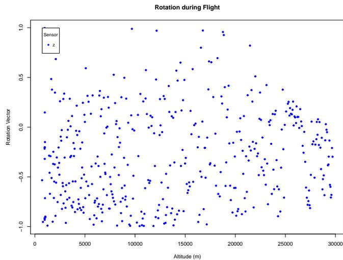
Figure 25: Rotation-altitude graph showing spinning during flight.
