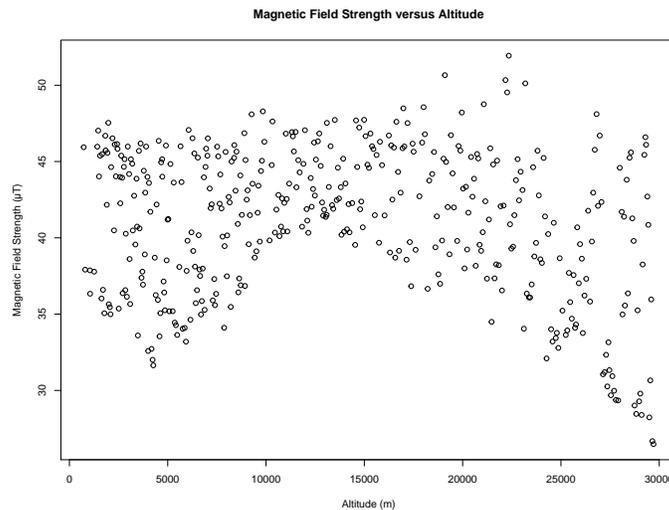
Figure 27: Magnetic field strength-altitude graph showing changes in the field during flight.
