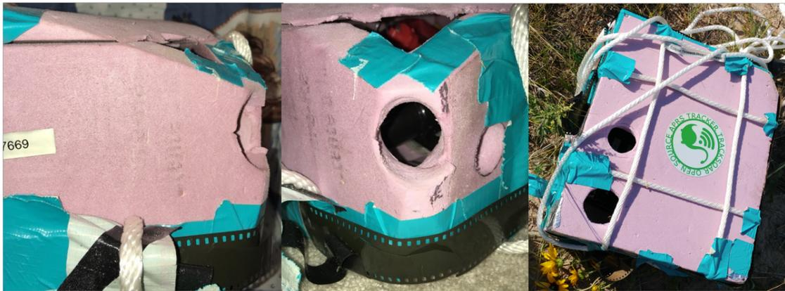
Figure 19: Corner designed not to impede the 360° view of the Gear camera.
