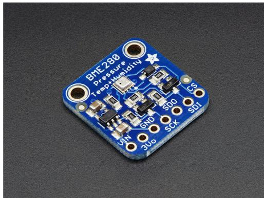
Figure 13: BME280 Sensor used by Tracksoar to measure temperature, pressure, and relative humidity.
