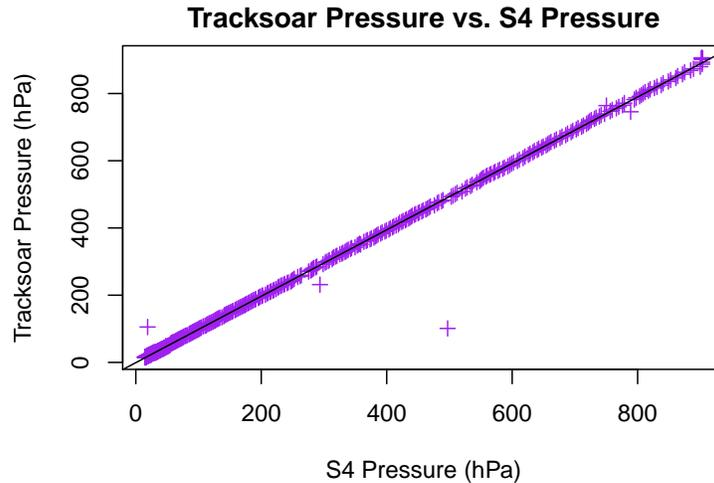
Figure 22: Pressure-pressure graph demonstrating the accuracy of the two pressure sensors.
