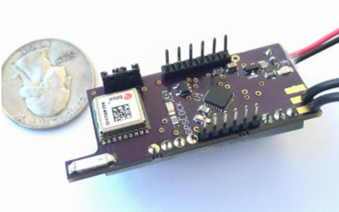
Figure 12: A Tracksoar APRS Tracking Device shown alongside quarter for scale. Antenna and battery not pictured.
