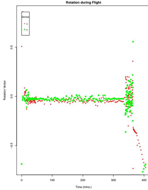
Figure 34: Rotation-time graph showing lack of swinging during ECLIPSE.
