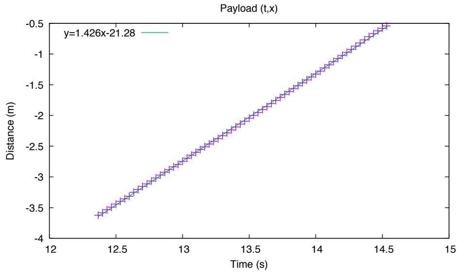
Figure 18: Position-time graph showing terminal velocity of TARC-16 parachute and dummy payload.
