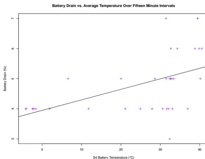
Figure 10: Graph of battery drain vs. average temperature over 15 minute intervals.
