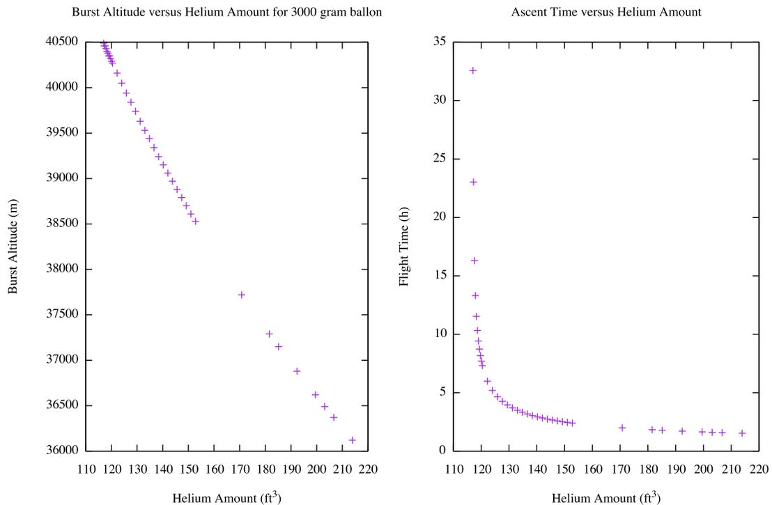
Figure 17: Graphs of ascent time and burst altitude, respectively, versus amount of helium.
