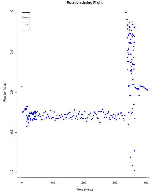
Figure 35: Rotation-time graph showing lack of spinning during ECLIPSE.
