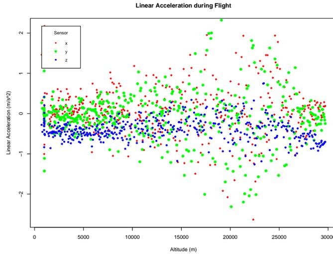
Figure 23: Acceleration-altitude graph showing three-axis acceleration during flight.
